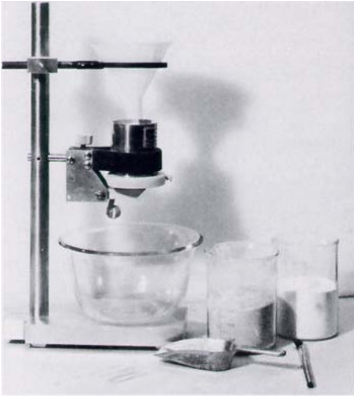
Figure 2: When loading is completed, 30 sec should be allowed for possible formation of individual flocculi or mass flocculation of the whole load.
